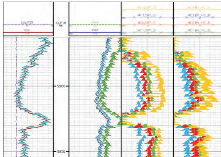
**Quantified uncertainty on output bulk volume hydrocarbon column has resulted from four different petrophysical modules.**
